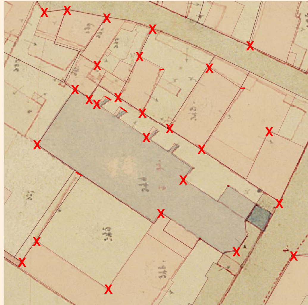
Thin plate spline georeferencing, e_{\max} > 1 \text{ m}
